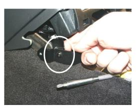
Attach frame support bracket (#4) to vehicle using 10/32 x ½" phillips machine screws, washers, and keps nuts
